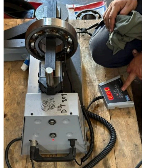
Figure 39 Heating Bearing with Electromagnetic Induction
