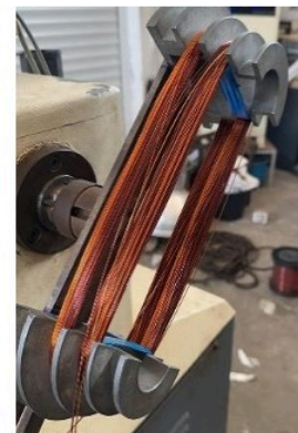
Figure 38 AC motor Coil making
